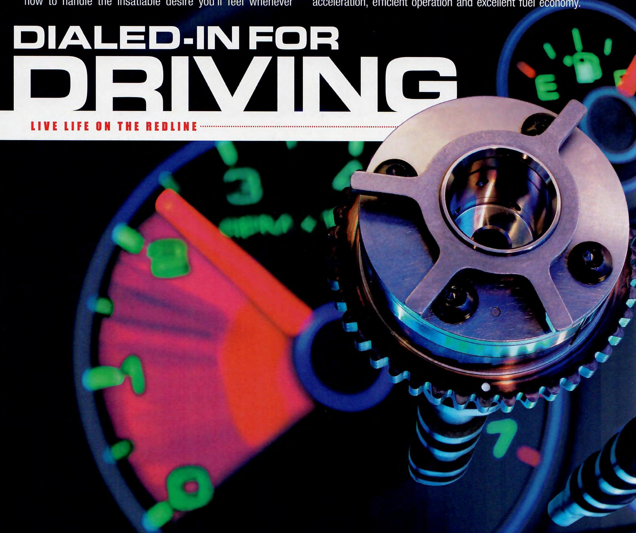
Both Fusion engines feature intake Variable Cam Timing (iVCT) for improved performance and efficiency. Unlike fixed valve timing - which achieves peak efficiency only when you hit the sweet spot at certain rpm - Fusion's iVCT continually adjusts intake valve timing to ensure the most complete and efficient combustion at a wider range in the rpm band. This enhances both low-end torque and high-rpm power. And what driver doesn't crave more of that?
